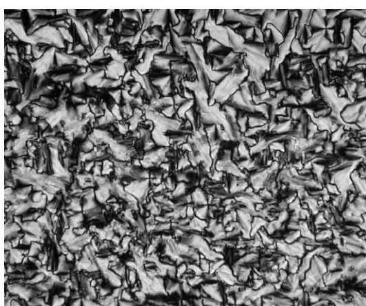
Figure 5. Typical texture of the monodendron 3 at 60 °C on cooling. Magnification: \times 200 .
